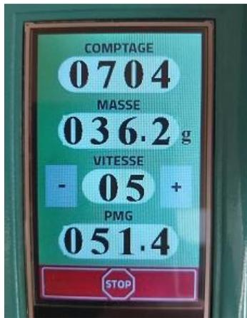
➤ *Digital display of number of grains (here, counting in progress) and the TGW.*
