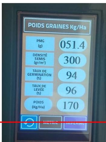
> *Integrated sowing simulator display: The user can display their sowing density objective in grains/m<sup>2</sup>,*
